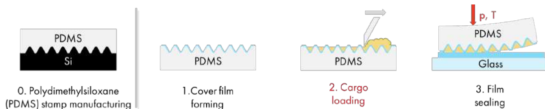
Figure 2.16: Process of manufacturing of MCA film.
