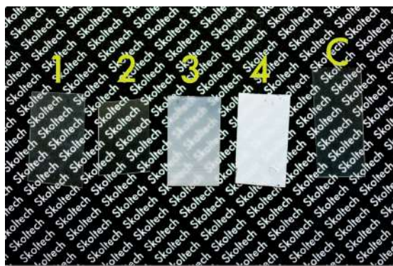
Figure 4.38: Irradiated PLGA films and control (non-irradiated) sample after 1-4 week incubation in PBS.
