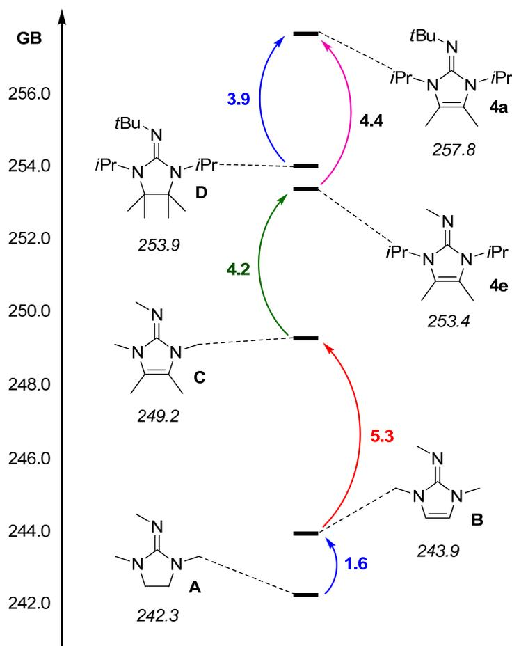
**Figure 3.5.** Calculated gas phase basicities (kcal mol<sup>-1</sup>) for imidazol-2-ylidene amines and their saturated analogues.
