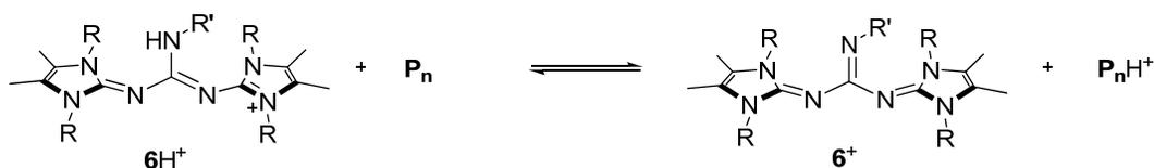
**Scheme 4.9.** Proton transfer equilibrium between BIG bases **6** and *t*BuP<sub>1</sub>(pyrr) and *t*BuP<sub>2</sub>(dma) bases (**P<sub>n</sub>**).
