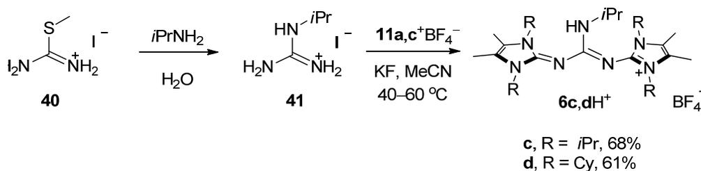
**Scheme 4.7.** Synthesis of alkyl substituted BIG salts  $6\text{c,dH}^+\text{BF}_4^-$ . Yields over two steps are given.
