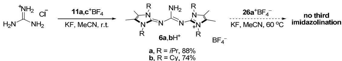
**Scheme 4.6.** Imidazolation of guanidinium chloride with formation of BIG salts  $6\text{a,bH}^+$ .
