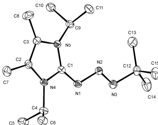
**Figure 2.1.** X-ray crystal structure of the triazene **23a**. The displacement ellipsoids are drawn on 30% probability level. Hydrogen atoms are omitted for clarity. Selected bonds distances [Å] and angles [°]: N(1)-C(1) 1.3411(16), N(4)-C(1) 1.3638(15), N(5)-C(1) 1.3618(16), N(4)-C(2) 1.3951(16), C(2)-C(3) 1.3537 (18), N(5)-C(3) 1.4115(17), N(1)-N(2) 1.3617(15), N(2)-N(3) 1.2517(16), N(3)-C(12) 1.4856(18).
