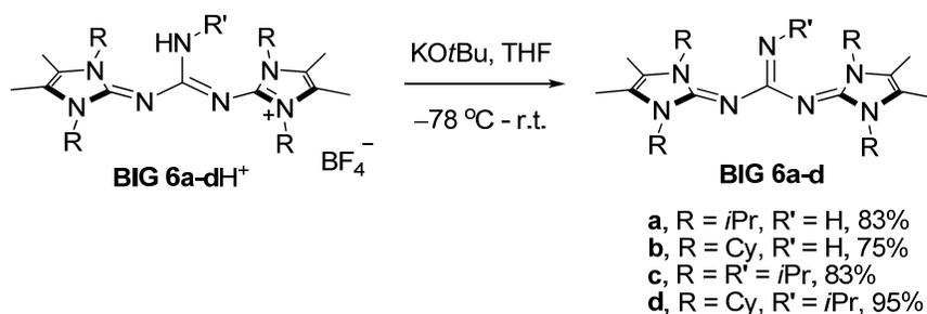
**Scheme 4.8.** Liberation of BIG bases **6a-d** from corresponding salts **6a-dH<sup>+</sup>BF<sub>4</sub><sup>-</sup>**.
