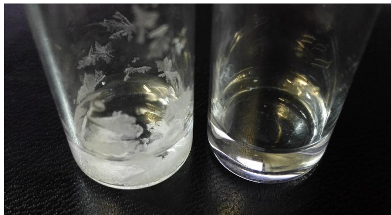
Figure 5.4. Mixtures of MeCN with a) [EMImOH]Cl (1M, left); b) [EMImOH]Cl + EG (1M and 2M respectively, right).
